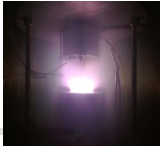
Figure 2. Plasma state in sputtering process
